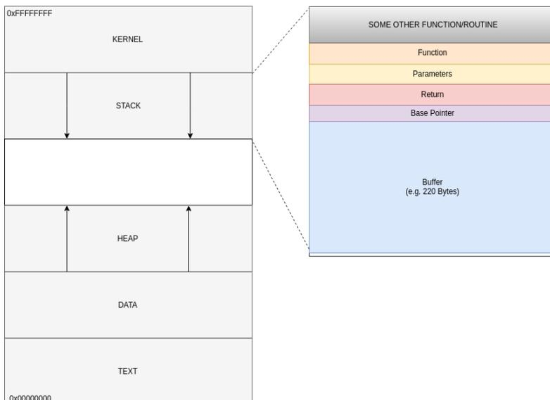
Figure 1 - Representation of Stack in Process Memory
